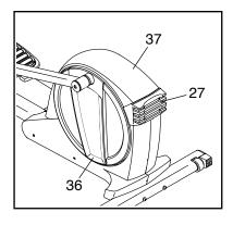
and then use a standard screwdriver to pry the Top Shield upward off the elliptical. Then, pry the left Pedal Disc (36) off the elliptical.
