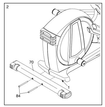
With the help of another person, place some packing inserts from the packing material under the front of the Frame (1) so that the Frame is lifted off the floor. Have another person hold the elliptical to prevent it from moving until this step is completed.
