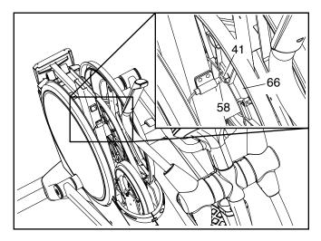
Next, slightly loosen the two indicated M4 x 16mm Screws (61). Slide the Reed Switch (58) slightly toward or away from the Magnet (41). Then, retighten the Screws.
