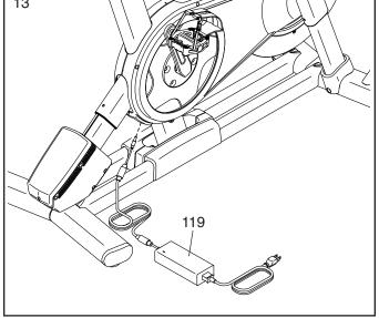
14. After the studio cycle is assembled, inspect it to make sure that it is assembled correctly and that it functions properly. Make sure that all parts are properly tightened before you use the studio cycle. Extra parts may be included. Place a mat beneath the studio cycle to protect the floor.
