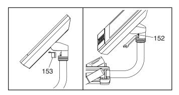
If the console feels too loose or does not stay in place when it is tilted upward and downward, **first see assembly step 8 on page 10.** Use a standard screwdriver to pry off the Console Covers (154, 155).
