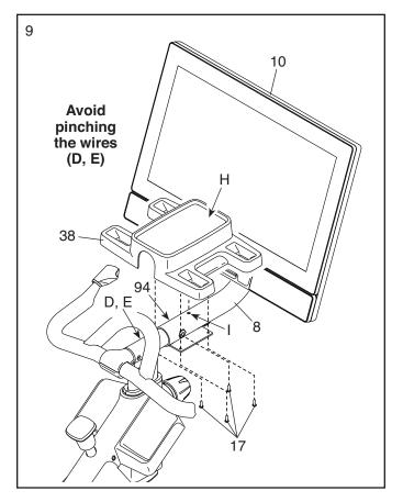
10. Position the wires (D, E) so that they fit neatly in the underside of the Hand Weight Tray (38).
