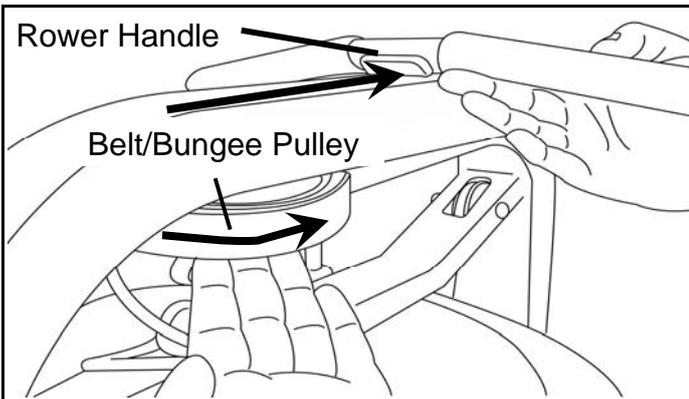
3. Wind the Rower Belt onto the Belt/ Bungee Pulley until the Rower Handle is as it's furthest forward position.
