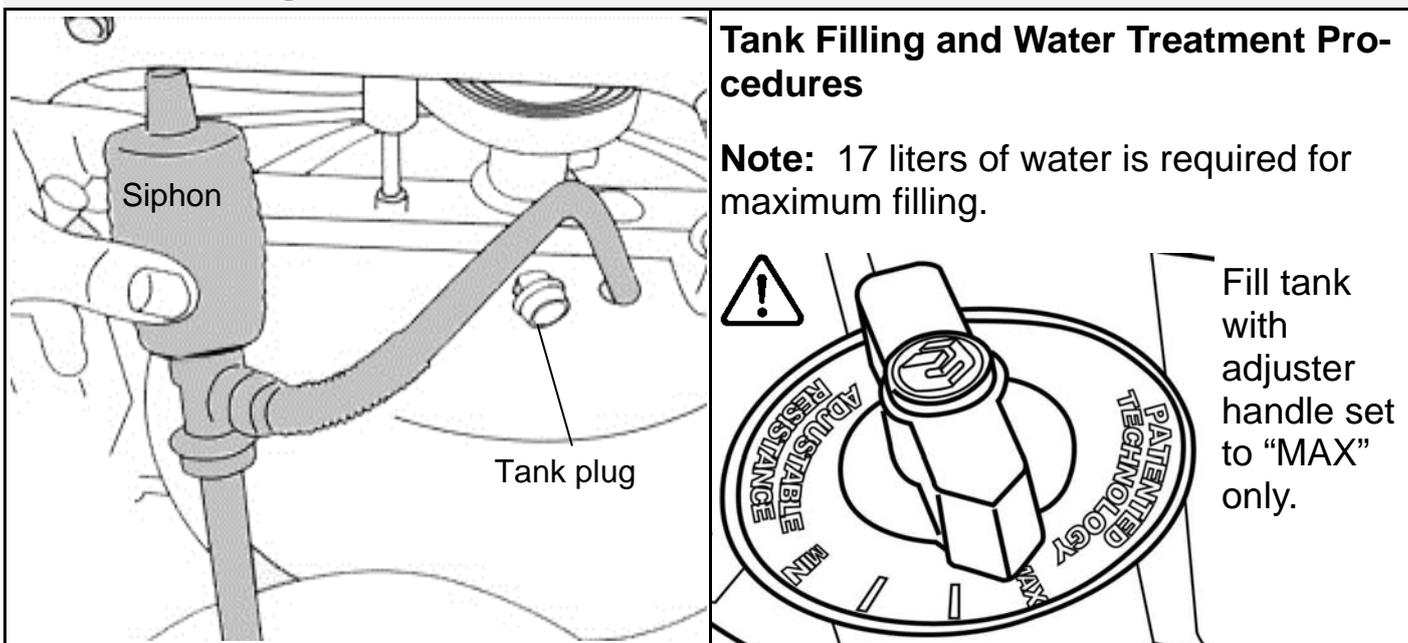
1. Remove Rubber Fill Plug from the top of the tank.
