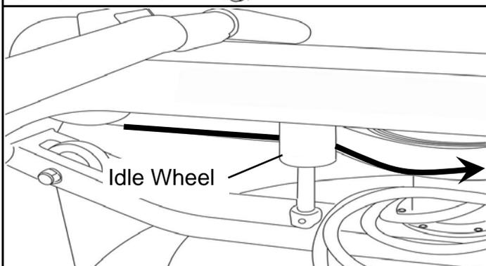
2. Next, thread the Belt around the Idle Wheel as shown. Once around the Idle Wheel, attach the Rower Belt to the Belt/Bungee Pulley. There is an obvious "lip" at the attachment point.
