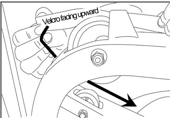
1. Begin reattaching the Rower Belt by threading around the Rower Belt Pulley with the Velcro side facing upward as illustrated.
