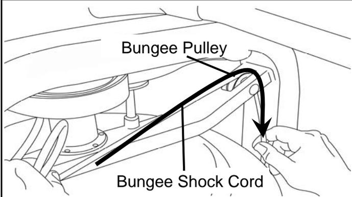
4. Rethread the Bungee Shock Cord (on opposite side of the Idle Wheel) back through the Bungee Pulleys and tie off at the Attachment Point.
