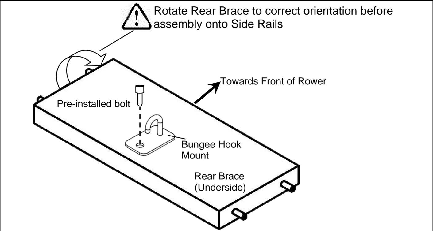
Next, connect the **Side Rail Left[2]** and **Side Rail Right[2]** using **4x M6x15mm Bolts[10]** and **Rear Brace[4]**. Do not tighten.
