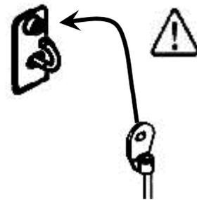
Do not cut Bungee tie wrap before Bungee cord is attached to rear of rower as shown here.
