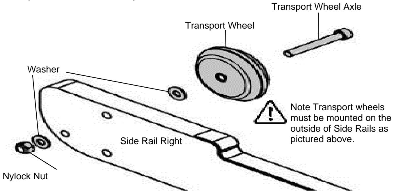
Once the Rear Brace and Side Rails are assembled, mount the Transport Wheel Assembly onto the Left/Right Side Rails.
