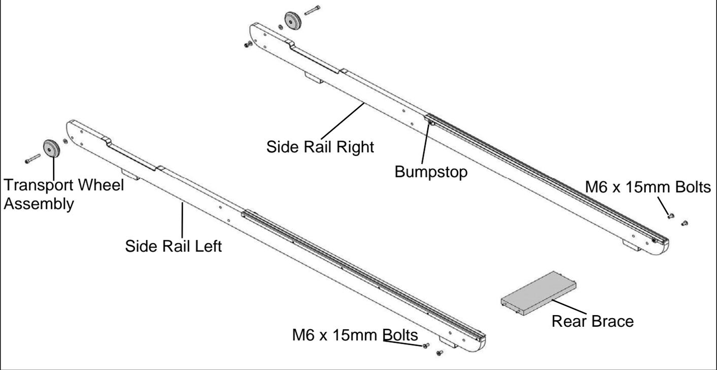
Tip: Bumpstops facing inside of rail for correct assembly orientation.
