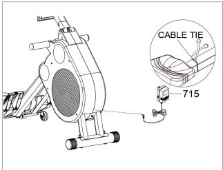
**Step 10:** Connecting the equipment to the mains supply
