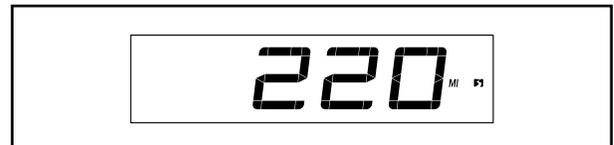
**Contrast Level**—The currently selected contrast level will appear in the display. Press the Silent Magnetic Resistance increase and decrease buttons to adjust the contrast level.
