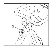
IMPORTANT: When the exercise bike is not in use, tighten the brake knob (G) completely.
