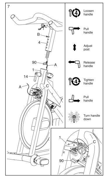
8. See the inset drawing. Connect the Upper Wire (90) to the Lower Wire (82). Tip: The wire connectors should slide together easily and snap into place with an audible click. If they do not, turn one connector and try again.
